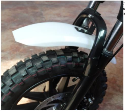
the bolt through the mudguard racket on to front fok and it.
