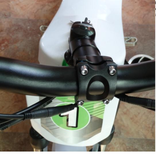
lebar in the bottom clamp, upper clamp on the install the 4pcs bolt
