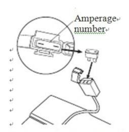
Remove the fuse and replace with a new one of equalamperage. Requires 30 ampfuse. Close the fuse cover andreattach the batery cover.
