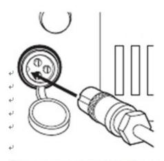
2 Turn power **OFF** before charging. Plug the charger into the charger port to charge unit.
