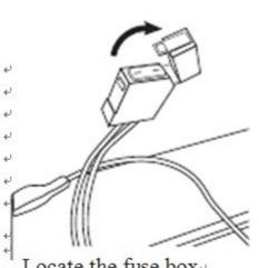
Locate the fuse boxe attached to the batteries. Opene the fuse cover to expose thee fuse.
