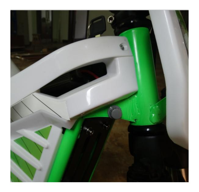
The speed limit switch is located the right side of front fork behind the front number plate. The switch,can control the speed from the lowest speed 5KMph to the high speed 35 KMph as end user's deminds.
