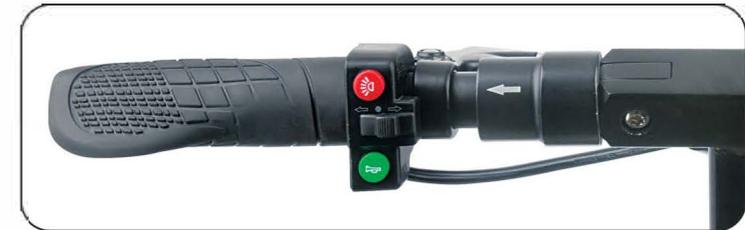
LEDfront light/speed control switch (left fast right slow)/horn switch
