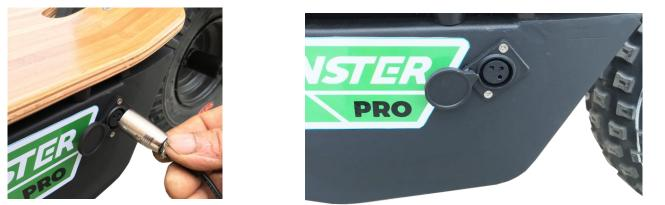
Finally fully charge your scooter before its first use. Charge it until the red light on the charger turns green. After it is finished charging remove the charger. Charge your scooter after every use. Never let it go completely dead and never charge it for any longer than 24 hours.
