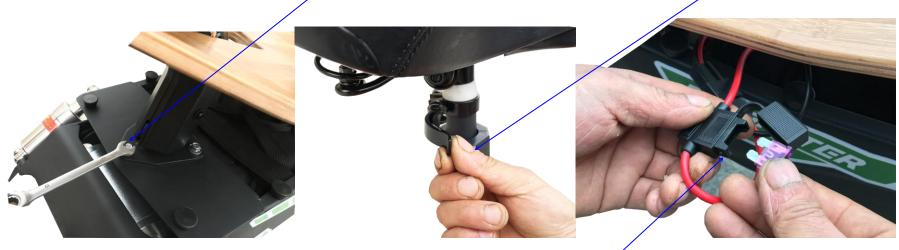
Put the fuse into battery box before you use the scooter.
